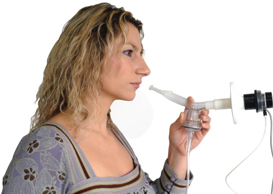
DeVilbiss 646 Nebulizer for integrated dosimetry tests
